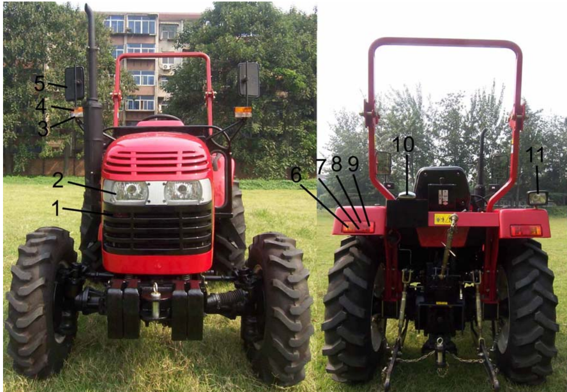
Fig.6-37 Distribution of lamplight and signal
