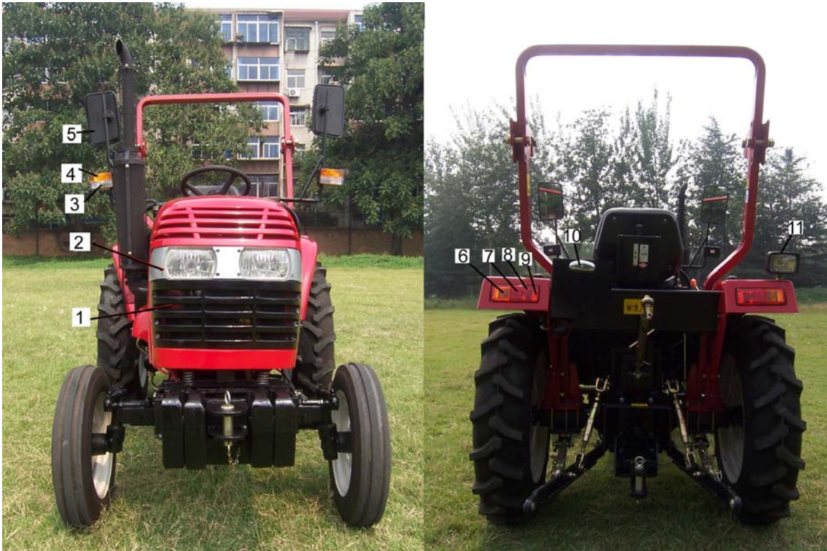
Fig 6-37 distribution of indicators and lights
